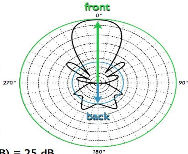
In this example the f/b ratio is:  $0 \text{ dB} - (-25 \text{ dB}) = 25 \text{ dB}$
