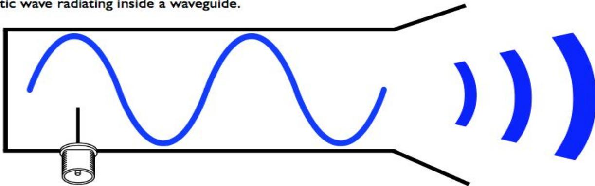
4. The wave leaves the waveguide and radiates mostly in one direction.
