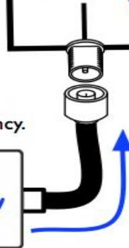
3. The wave arrives at a bare wire, and induces an electromagnetic wave radiating inside a waveguide.
