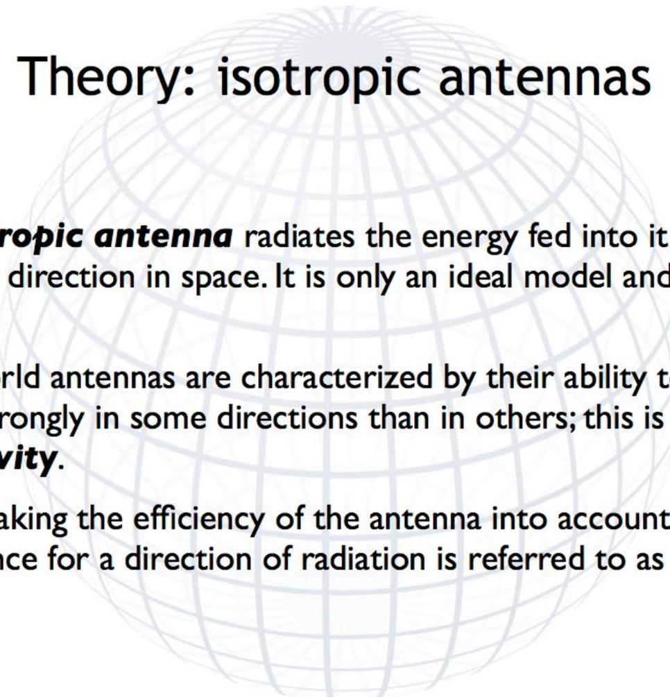
An **isotropic antenna** radiates the energy fed into it equally in every direction in space. It is only an ideal model and cannot be built.
