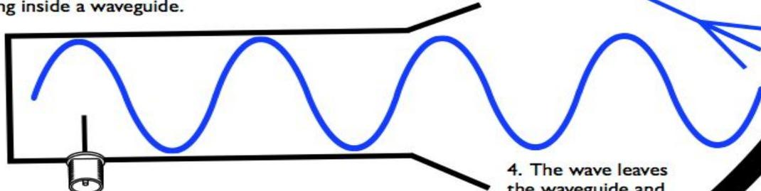
4. The wave leaves the waveguide and radiates towards a reflector.
