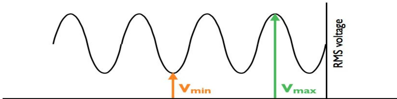
$$\text{Voltage Standing Wave Ratio VSWR} = \frac{V_{\max}}{V_{\min}}$$
